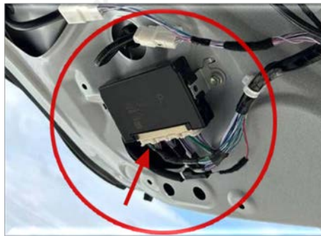
Connecting with needles to MND ECU in the trunk (tailgate)
