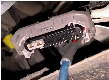
Connecting with needles to Headlight ECU
